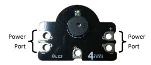
The spare power port can be used to pass electricity on to other devices.
