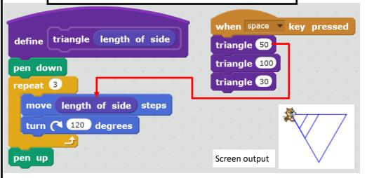
When the space key is pressed the **adaptable triangle procedure** will draw three triangles. The number will be used by the procedure as the length of the sides.
