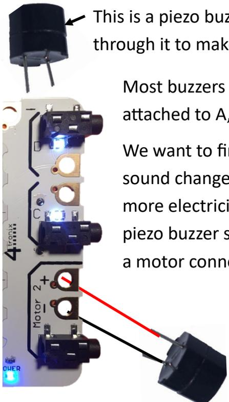
This is a piezo buzzer. We pass electricity through it to make sounds.
